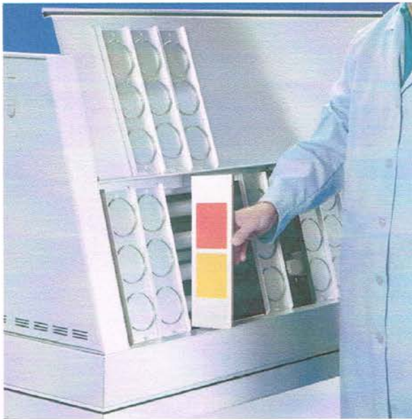
Test specimens are mounted on both the front and back side of the QUV, providing a large sample capacity.
