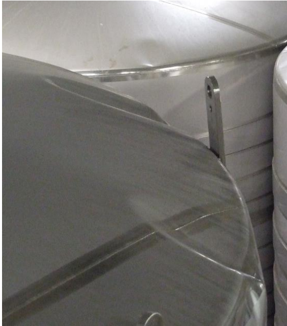
Roof buckling from pressurisation
