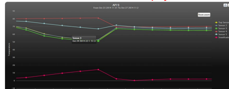
Visualise thermal stratification of an entire ferment
